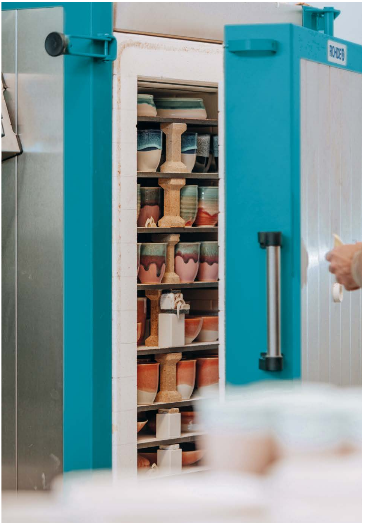
A chamber kiln from the KE-N series – 480-litre firing chamber heated with electricity from photovoltaics.
