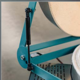
Gas pressure spring for easy and safe lid opening
